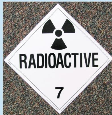
Seems like something is missing on this Class 7 Radioactive Placard? Can you find what is wrong easily? Is a yellow triangle in the upper portion of a class 7 placard required to be there? Should you always inspect your shipping communications before use? Will the manufacturer or the shipper be held responsible for using a placard that does not fully meet the required specifications in 49 CFR 172 Subpart F? I appreciate the folks who shared this placard with me during training. Thank you!
