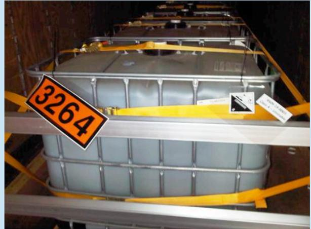
Where should you apply your 'package' specification communications? Is the shoring bar considered part of the package and a good location for the Orange Panel? Or is the web tiedown a better place for package communications, like the Class 8 corrosive label and other package markings? I hope you said the package communications should go physically on the package or in this case, the portable tank.
